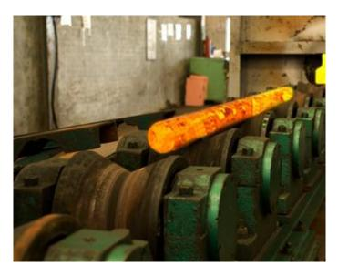
Hot Mill for the Manufacturing of Seamless Mother Hollows
