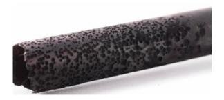
Under metal dusting conditions, vulnerable materials are disintegrated in high amounts of coke mixed with metal, metal carbides and metal oxides.
